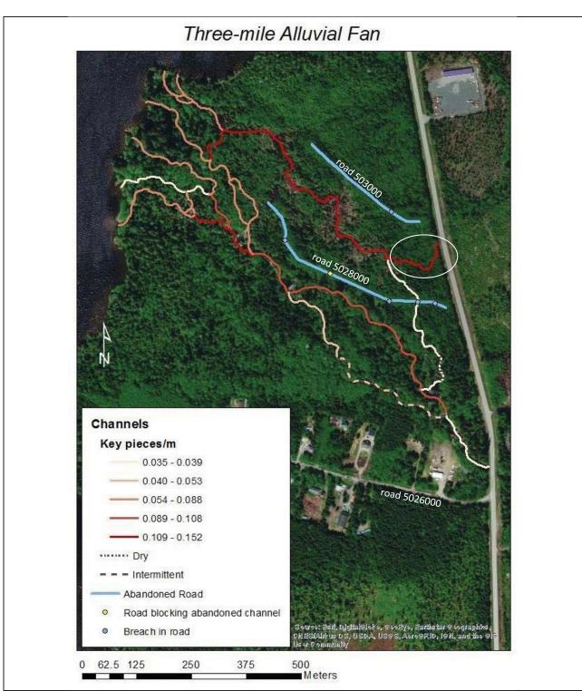
**Figure 1.** Active channels in the alluvial fan, density of key pieces of wood in different reaches, and abandoned (blue lines) and open roads. Note that the small northern tributary (in circle) flows through a culvert under the highway, but was only mapped downstream of the highway.
